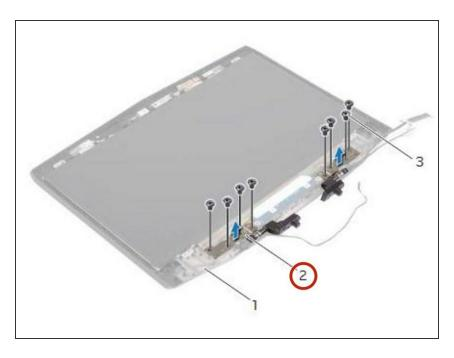
Remove the display hinges off the display back-cover.
