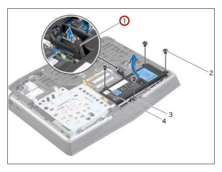
Connect the battery cable to the system-board connector.
