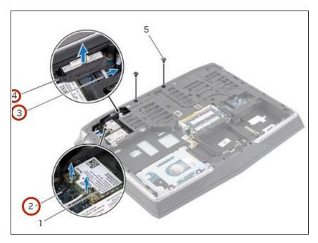
Remove the display, camera, and antenna cables from the slots on the computer base.
