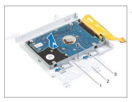
Turn the secondary hard-drive assembly over.
