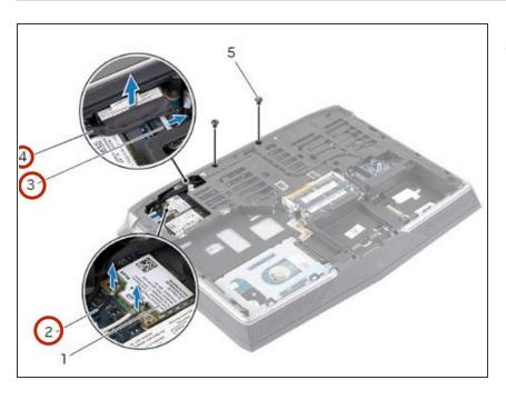
Route the display, camera, and antenna cables through the routing guides.
