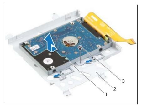
Replace the screw that secures the secondary hard-drive assembly to the main bracket.
