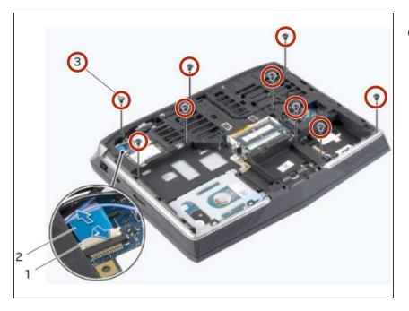
Remove the screws that secure the palm -rest assembly to the computer base.
