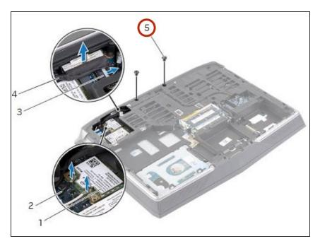
Replace the screws that secure the display assembly to the computer base.
