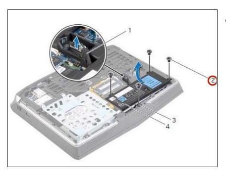
Remove the screws that secure the battery to the computer base.
