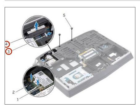
Connect the display and camera cables to the system-board connectors.
