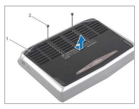
Align the tabs on the NEW base cover with the slots on the computer base and slide the base cover into place.
