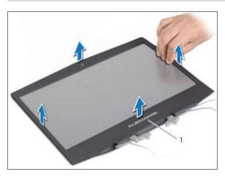
Align the **NEW** display bezel with the display back-cover, and gently snap the display bezel into place.
