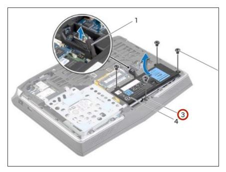
Align the tabs on the **NEW** battery with the slots on the computer base.
