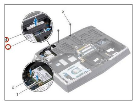
Disconnect the display and camera cables from the system-board connectors.
