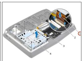
Carefully lift the secondary hard-drive assembly and then lift the latches to release the secondary hard-drive cable from the system-board connector.
