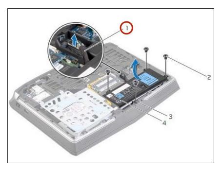
Using the battery cable, lift the battery and release it from the tabs on the computer base.
