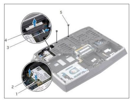
Slide the cables through the slots on the computer base.
