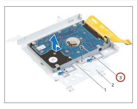
Remove the screw that secures the secondary hard-drive assembly to the main bracket.
