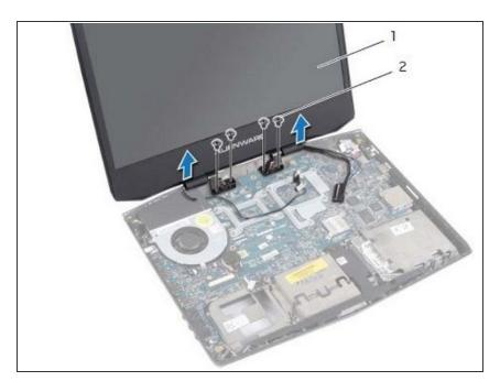
Note the display, camera and antenna cable-routing and remove the cables from their routing guides.
