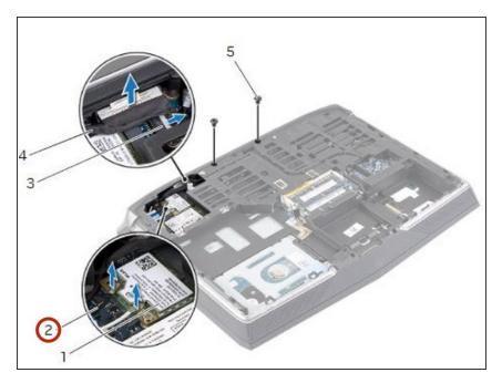
Connect the antenna cables to the wireless mini-card.
