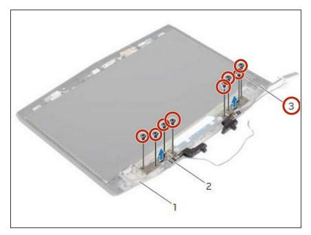
Align the screw holes on the NEW display hinges with the screw holes on the display back-cover.
