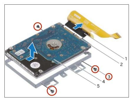
Remove the screws that secure the secondary hard-drive to the secondary hard-drive bracket.
