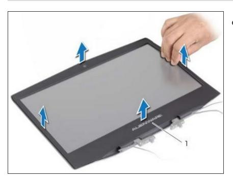
Remove the display bezel off the display back-cover.
