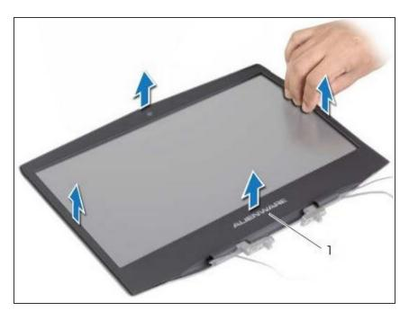
Align the **NEW** display bezel with the display back-cover, and gently snap the display bezel into place.
