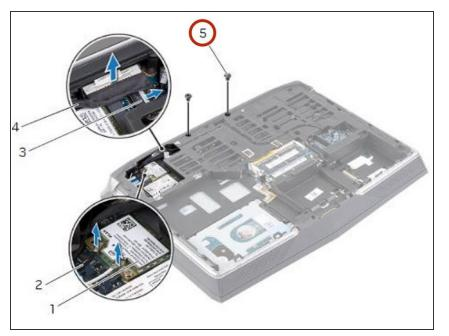
Remove the screws that secure the display assembly to the computer base.
