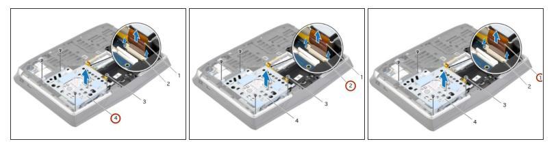
• Carefully lift the secondary hard-drive assembly and then lift the latches to release the secondary hard-drive cable from the system-board connector.
