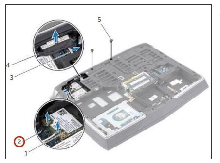
• Connect the antenna cables to the wireless mini-card.
