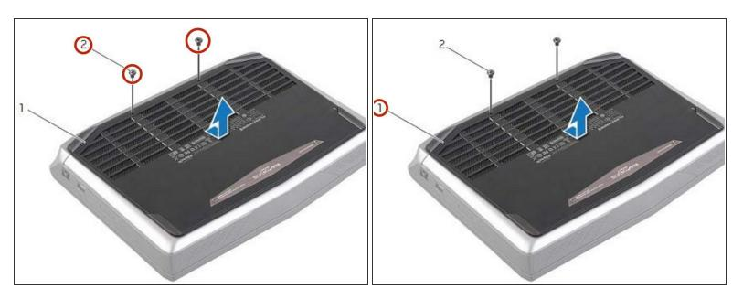
• Remove the screws that secure the base cover to the computer base.
