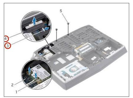
Connect the display and camera cables to the system-board connectors.
