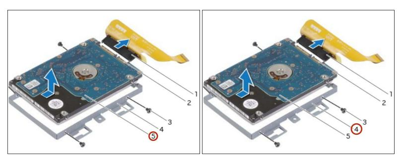
• Slide and lift the secondary hard-drive off the secondary hard-drive bracket.
