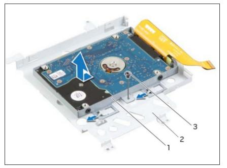
Place the NEW secondary harddrive in the secondary hard-drive bracket.
