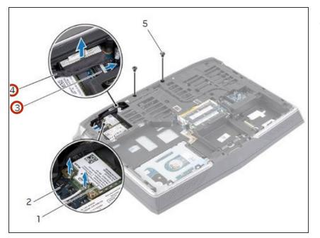
Disconnect the display and camera cables from the system-board connectors.
