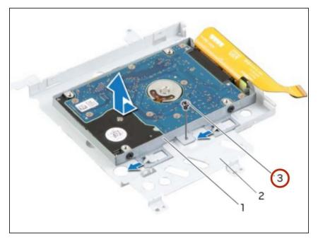
• Align the screw hole on the secondary hard-drive assembly with the screw hole on the main bracket.
