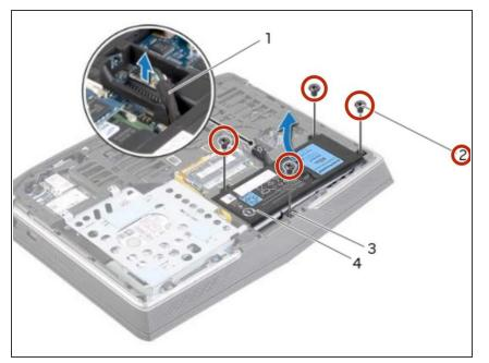
• Replace the screws that secure the battery to the computer base.
