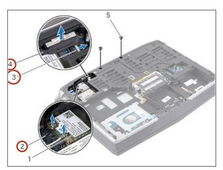
Slide the cables through the slots on the computer base.
