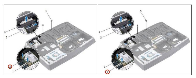
Disconnect the antenna cables from the wireless mini-card.
