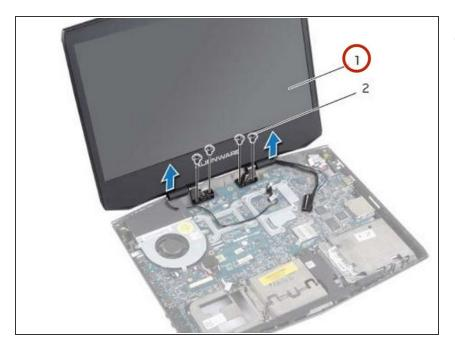
• Lift the display assembly off the computer base.
