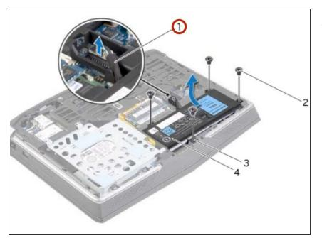
• Connect the battery cable to the system-board connector.
