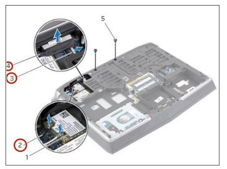
Remove the display, camera, and antenna cables from the slots on the computer base.
