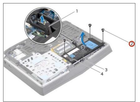
Align the screw holes on the battery with the screw holes on the computer base.
