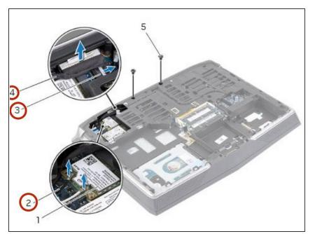
Route the display, camera, and antenna cables through the routing guides.
