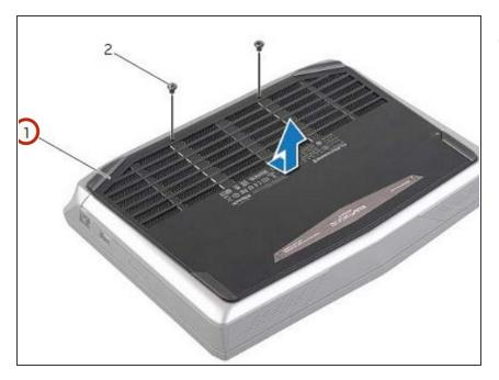
• Slide and lift the base cover off the computer base.
