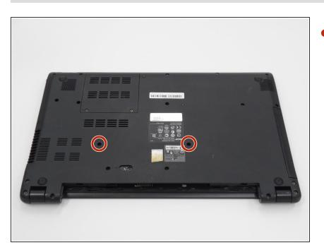
• Remove the two 6mm PH1 screws from the bottom of the laptop.
