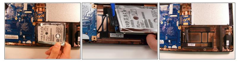
• Lift the HDD out of the base and use the opening tool to disconnect the HDD from the motherboard wire.
