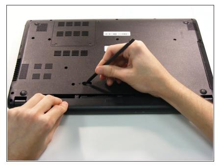
Use the pointed end of the spudger to slide the battery lock until the battery pops loose.
