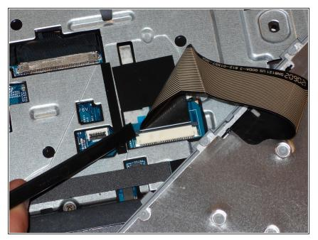
• Use the spudger and slide the grey tabs on either side of the keyboard wires away from the white plastic.
