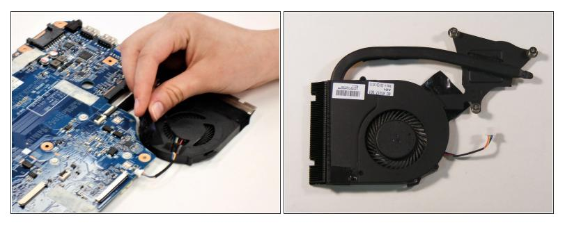
On the side opposite the CPU fan screws, pull loose the tape securing the fan assembly to the motherboard.
