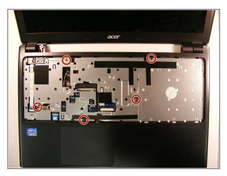
• Remove the five 6mm PH1 screws beneath the keyboard.
