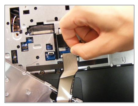
• Disconnect the keyboard by pulling the blue tape on the wire strip.
