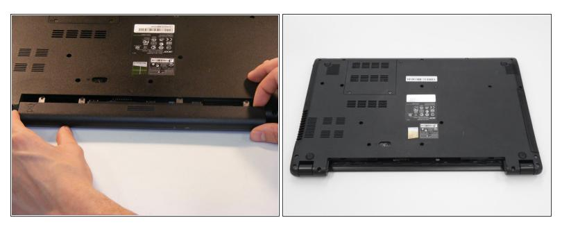
• Slide the battery out of the battery slot.
