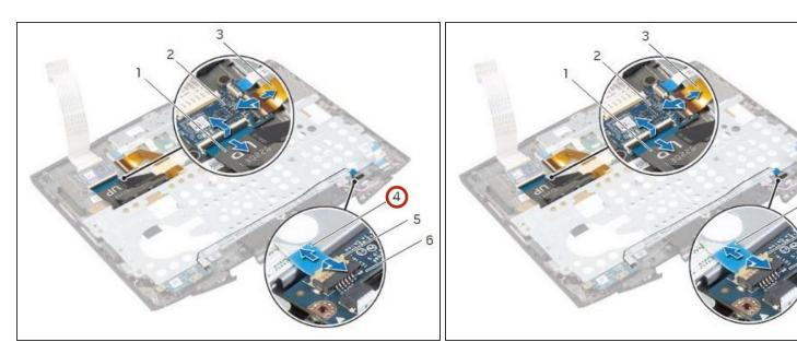
Slide the power-button board cable into the status-light board connector and press down on the connector latch to secure the cable.
