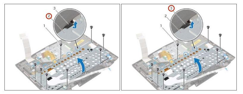
Slide the keyboard bracket under the tabs on the palm-rest assembly and align the screw holes on the keyboard bracket with the screw holes on the palm-rest assembly.
