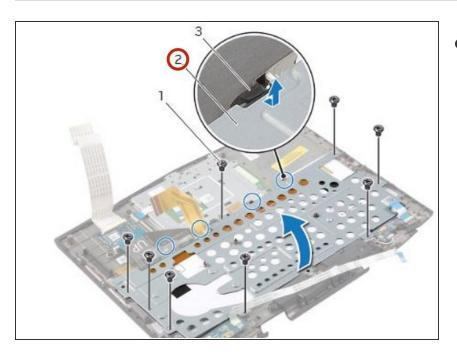
Lift the keyboard bracket off the keyboard.
