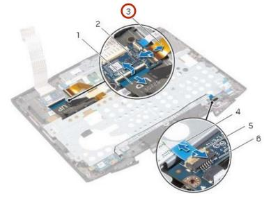
Slide the keyboard cable and keyboard-backlight cable into the keyboard-board connectors and press down on the connector latches to secure the cables.
