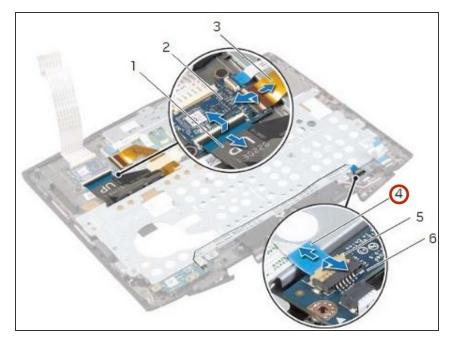
Peel the power-button board cable off the keyboard bracket.
