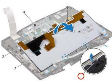
Lift the keyboard and release it from the tabs on the palm-rest assembly.
