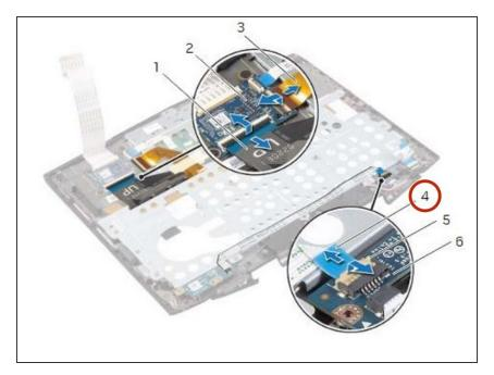
Route the power-button board cable on the keyboard bracket and adhere the cable to the keyboard bracket.
