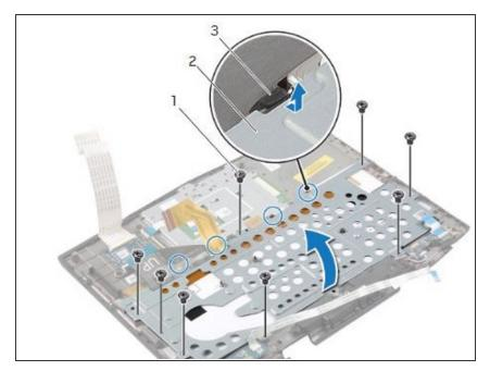
Slide the keyboard cable and keyboard-backlight cable through the keyboard bracket.
