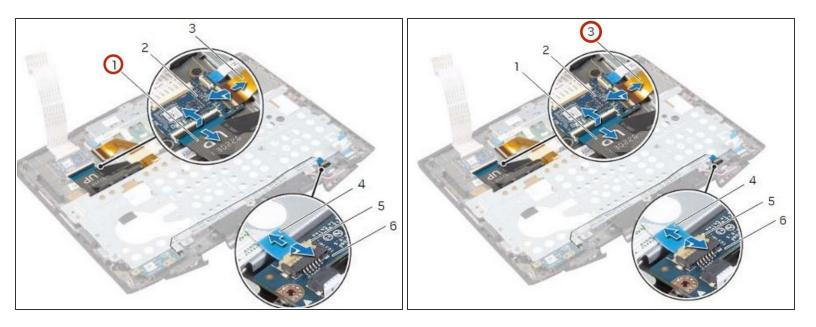
Slide the keyboard cable and keyboard-backlight cable through the keyboard bracket.
