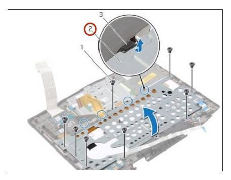
Lift the keyboard bracket at an angle and release it from the tabs on the palm-rest assembly.
