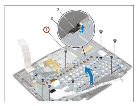
Remove the screws that secure the keyboard bracket to the palm-rest assembly.
