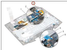
Lift the connector latches and disconnect the keyboard cable and keyboard-backlight cable from the keyboard-board connectors.
