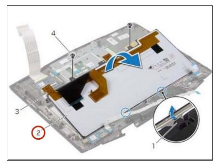
Slide the **NEW** keyboard under the tabs of the palm-rest assembly and align the screw holes on the keyboard with the screw holes on the palm-rest assembly.
