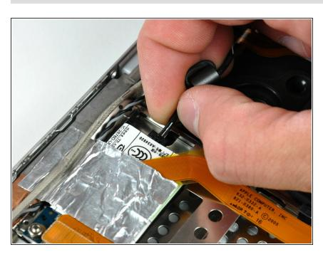
Disconnect the RJ-11 cable from the modem.
