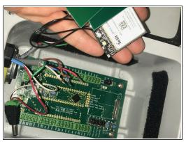
Pull the module from the bottom; pulling the module in a different way may damage it
