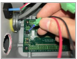
To disconnect the blue circled point on the solar charger, you have to remove the terminal at the blue circle on the board
