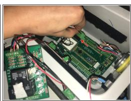
(i) If you choose to disconnect the wires from the terminal, we recommend you either write down the wires' respective locations on the terminal, or consult our pin documentation when reassembling
