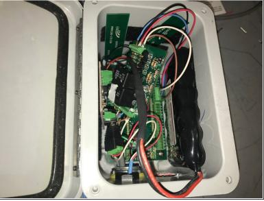
(i) Generally, there will also be ultrasonic components, such as wires, present within the node. There is no ultrasonic connected to our node in order to focus entirely on the autosampler
