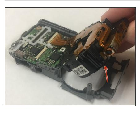
Gently lift and remove the lens casing, pulling it free from the now disconnected ribbon cable. To reassemble your device, follow these instructions in reverse order.
