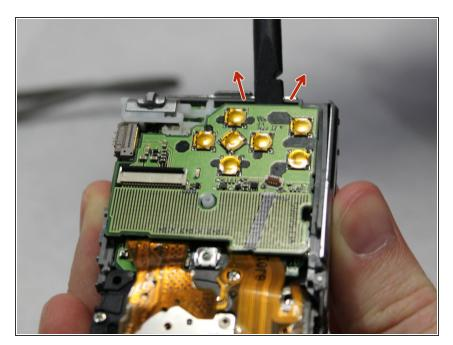
Insert the flat end of a spudger underneath the motherboard and twist. This will disconnect it from the rest of the device.
