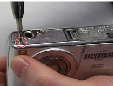
Remove both of the 3 mm screws on the bottom of the camera connected to the side panel.
