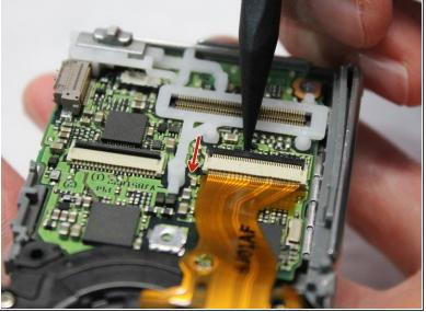
• Using the pointed end of a spudger, flip up the two black tabs holding the ribbon cables in place.
