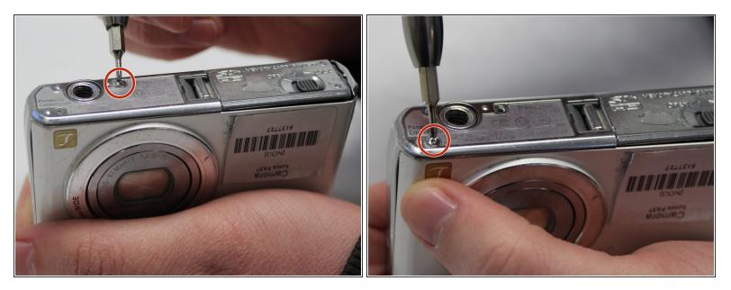
• Remove both of the 3 mm screws on the bottom of the camera connected to the side panel.
