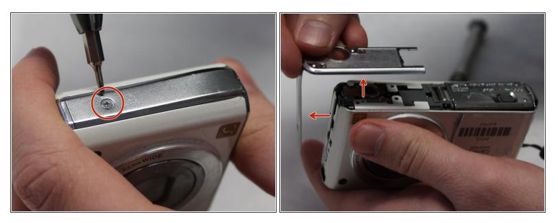
• Remove the remaining 3 mm screw holding on the side panel and remove the panel entirely.
