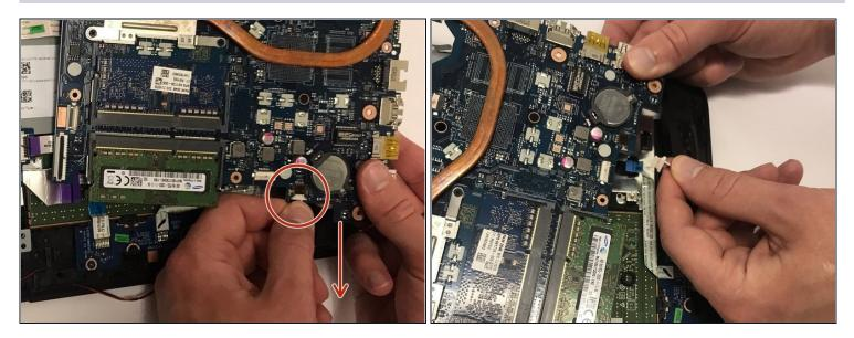
• Pull out the white cable (contains red and white cable attached to a black support) with wires from its port.
