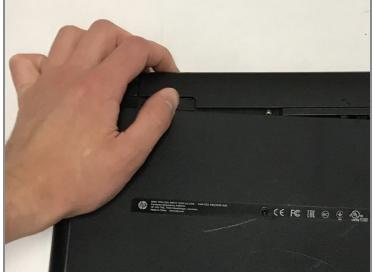
• To remove the battery, slide the left slider on the back to the unlocked position.
