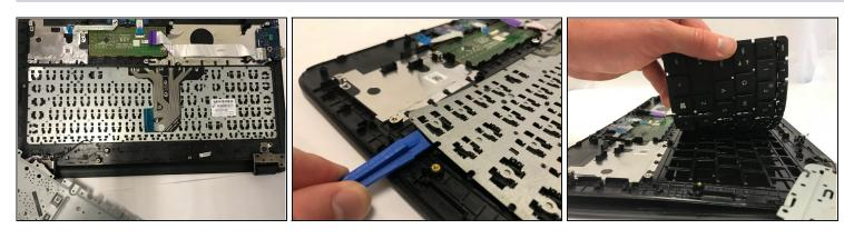
Locate the damaged keyboard and lift up with the prying tool to remove.
