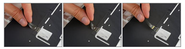
• Gently peel the keyboard ribbon cable up from the case, and remove the cable.
