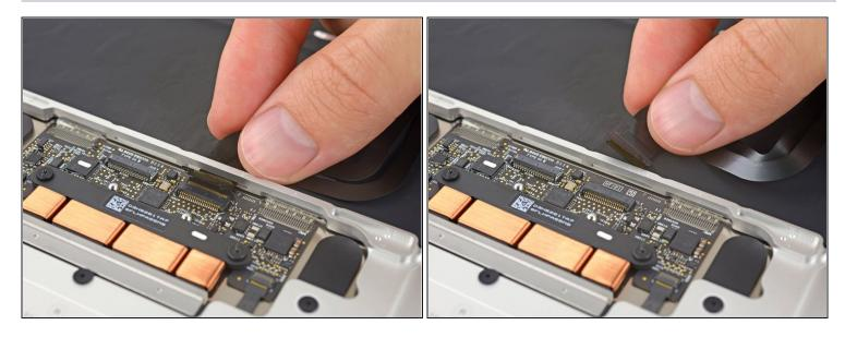
• Gently pull the keyboard ribbon cable out of its slot in the frame.
