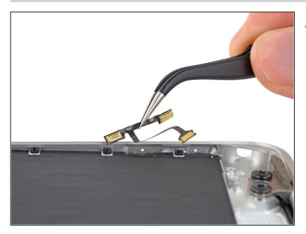
• Remove the dual microphone assembly.
