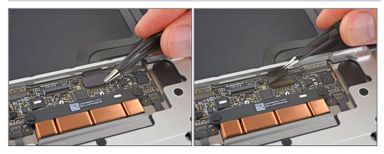
• Use a pair of <u>tweezers</u> to remove the tape covering the keyboard ribbon cable connector on the trackpad.
