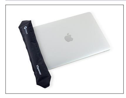
• <u>Prepare an iOpener</u> and apply heat to the upper case directly behind the microphone assembly.
