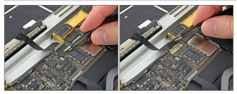
• Use <u>tweezers</u> to peel back the tape covering the display cable connector.
