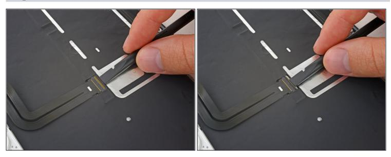
• Use a spudger to flip up the retaining flap on the keyboard ribbon cable ZIF connector.
