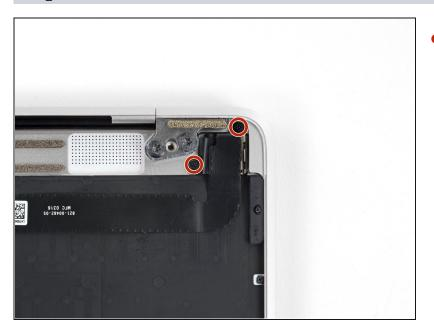
Remove two 2.5 mm Phillips #00 screws securing the USB-C port.
