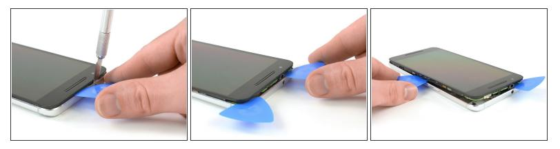
Insert a razor knife between the metal back cover and the front glass to create a gap. Insert an
