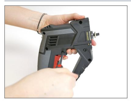
Flip over the rear body, and unscrew the 9 20mm screws.
