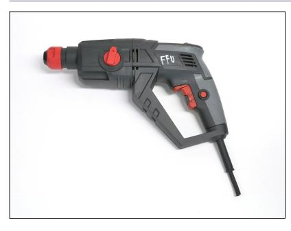
i The Skil 1743-AA Cordles SDS+ Hammer Drill is an affordable tool for serious hole drilling. Note that this one had its labels removed and the cord cut off for educational purposes.
