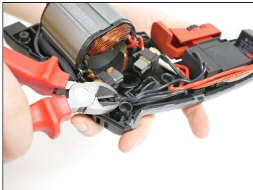
• With pliers, cut the cable ties that secure the cable tree.
