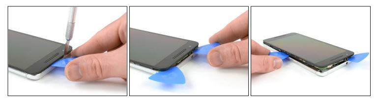
• Insert a razor knife between the metal back cover and the front glass to create a gap. Insert an opening pick into the gap and slide it to the top right corner.
