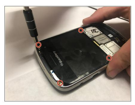
Using the T5 Torx Screwdriver, remove the four torx screws that are located on the bottom half of the device
