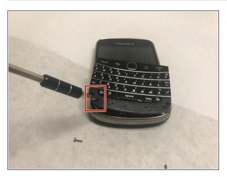
Now lever the keyboard up using the screwdriver in the indicated hole.
