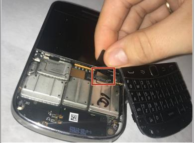
• The keyboard is attached via a ribbon cable. Pull the cable up to remove the keyboard.
