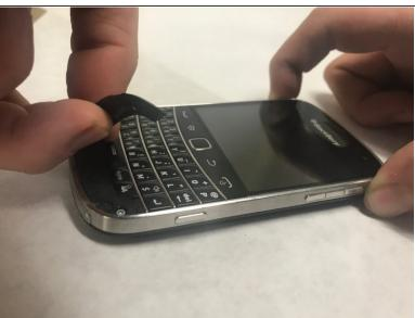
Lift the bezel at the bottom of the phone up and peel it away from the phone.
