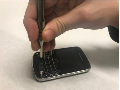
Remove the two exposed screws using the T5 Torx screwdriver.
