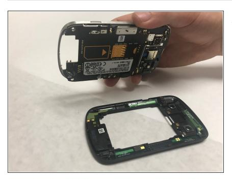
Now, carefully and gently using your fingers, lift and remove the assembly from the back case.
