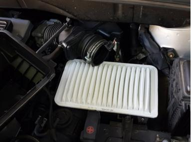
Replace the filter and assemble in reverse order.
