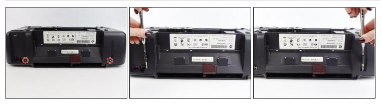
Remove the two 13 mm screws located on the back of the printer using a screwdriver with the T10 torx bit (star-shaped).
