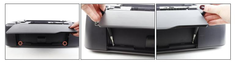
• In the front of the printer, open the tray where the paper comes out and remove the two 13 mm screws located under the top of the printer.
