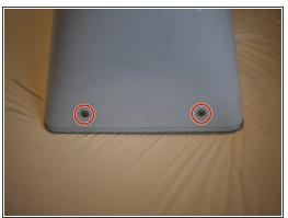
Remove two 2.5mm hex screws from each of the other sides of the computer.
