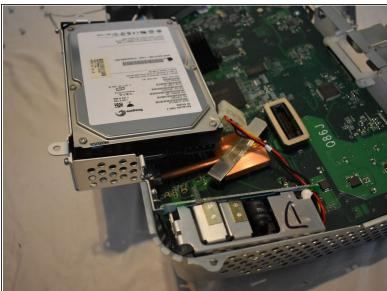
Disconnect the 4-pin hard drive power connector.
