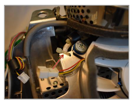
There may be a zip tie holding another cable to the fan assembly, cut it to remove the fan assembly.
