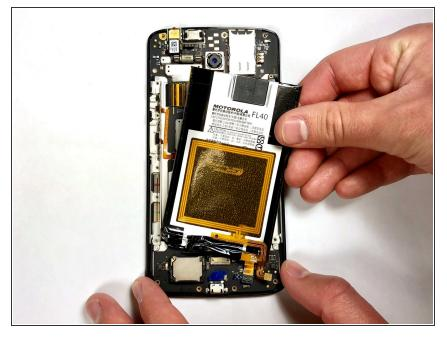
• Remove the disconnected battery from the phone.
