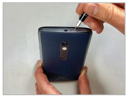
Insert a small pointed object into the hole on the sim card tray to eject the tray from the phone.
