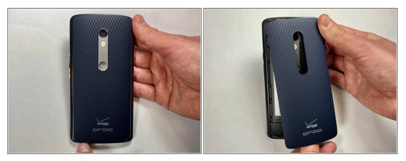
Wedge your thumb into the indent located on the bottom left corner of the back cover and pull up to remove the back cover.
