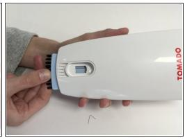
Remove the blue switchbutton from the upper part of the nozzle by putting a momentum on the edge. After you have done this signature move you can remove the brush.
