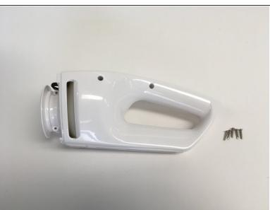
Remove 4 screws on the side and 1 screw on the bottom. You'll do this by crosshead screwdriver size number 1.
