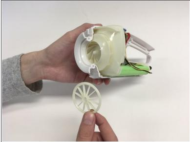
Remove the turbine protector in front of the turbine.
