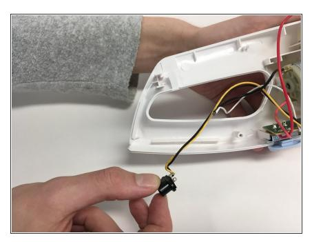
Pull the charge socket out of the plastic cover.
