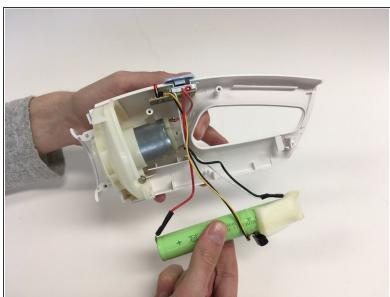
Pull the battery out. It still has some wires attached to it.
