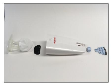
Right now the whole nozzle is disassembled, except for two small steel rings. These will break if you try to remove them.
