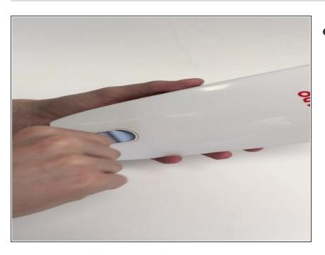
Remove the blue switchbutton from the upper part of the nozzle by putting a momentum on the edge. After you have this signature move you can remove the brush. You can see the video for the signature move.
