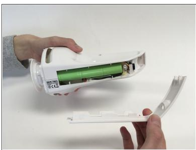
Remove the lid from the battery lid by sliding it and after pull it out.
