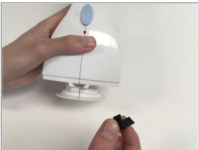
Remove the black clip from the inner top side of the body.
