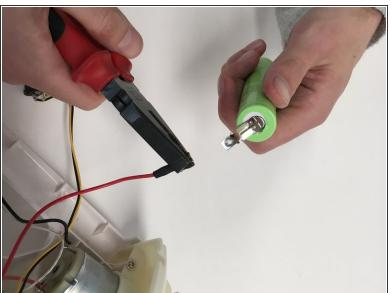
Use the pliers to remove the wires from the battery.
