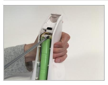
Remove the screw after removing the lid above the battery.
