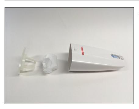
Remove the big parts that are inside of the nozzle. These parts consist of a plastic structure with a filter.
