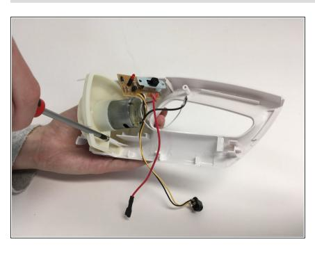
Remove the last screw with a number 1 screwdriver, next to the electro motor to release the motor + turbine.
