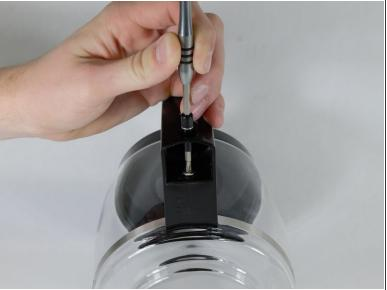
Use the bit driver with the Phillips PH1 bit to remove the 27 millimeter long screw in the base of the handle.
