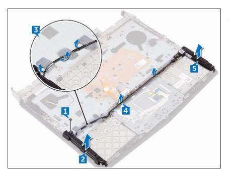
Peel off the tape that secures the speaker cable to the palm-rest assembly.
