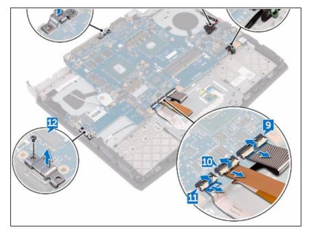
Remove the screw (M2.5x6L) that secures the USB Type-C port bracket to the system board and lift the USB Type-C port bracket off the system board.
