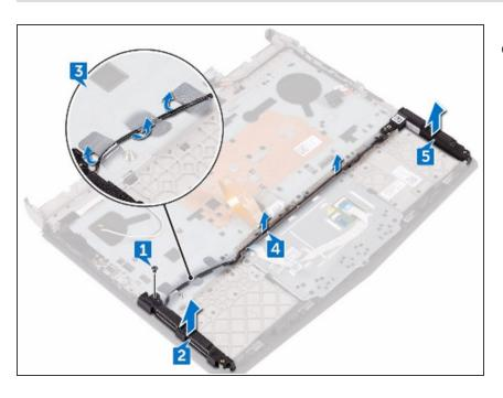
Using the alignment posts, place the NEW left speaker on the palm-rest assembly.
