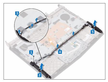
Replace the screw (M2x3) that secures the speaker to the palm-rest assembly.
