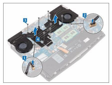
In sequential order (as indicated on the heat-sink assembly), remove the seven screws (M2x3) that secure the heat-sink assembly to the system board.
