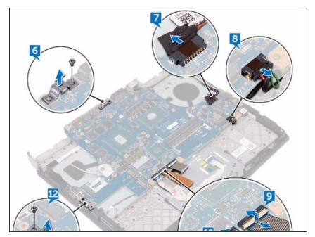
Replace the screw (M2.5x6L) that secures the USB Type-C port bracket to the system board on the back and right side of your computer.
