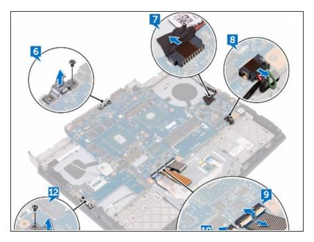
Open the latch and disconnect the keyboard cable from the system board.
