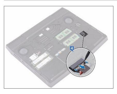
Using a plastic scribe, disconnect the battery cable from the system board.
