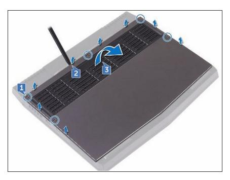
Slide the tabs on the NEW base cover into the slots on the computer base and snap the base cover into place
