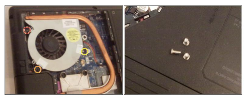
To remove the fan, remove the three screws that hold it into the system. Disconnect the fan before removing it.
