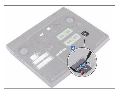
Using a plastic scribe, disconnect the battery cable from the system board.
