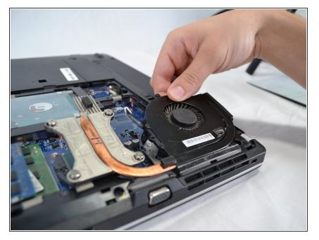
To remove the heatsink and fan, pull the fan upwards and towards the center.
