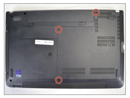
Remove the three 1.2mm Phillips #00 screws from the bottom panel.
