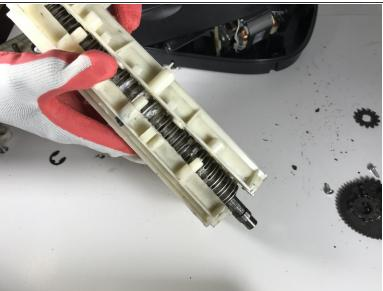
Replace the mill cutter paper stripper set and stripper guide set.
