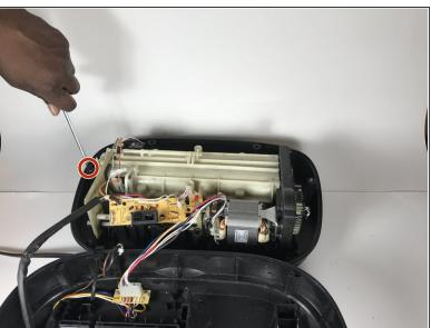
Remove the screws connecting the stripper guide and the base of the shredder's housing unit with a Phillips screwdriver. The diameter head and screws are 10 mm in length.
