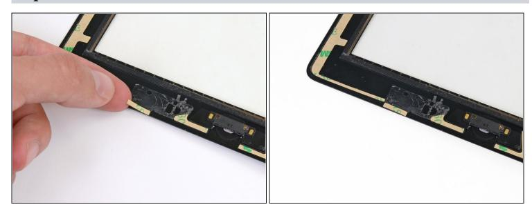
• Lay the final small rectangular adhesive strip to the left of the hook-shaped adhesive strip, immediately to the right of the thin L-shaped strip, and flush with the bottom of the front panel.
