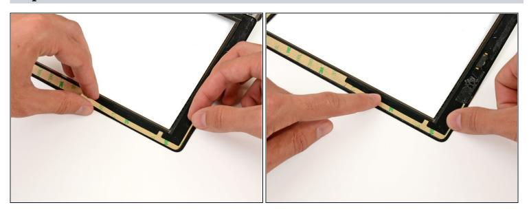
• Place the thinnest L-shaped adhesive strip on the bottom left corner of the front panel.
