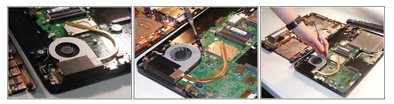
Using a Phillips #1 screwdriver, remove the one 1.5mm screw.
