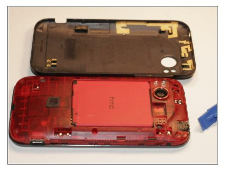
Use a plastic opening tool or your fingers to get into the groove between the cover and case.
