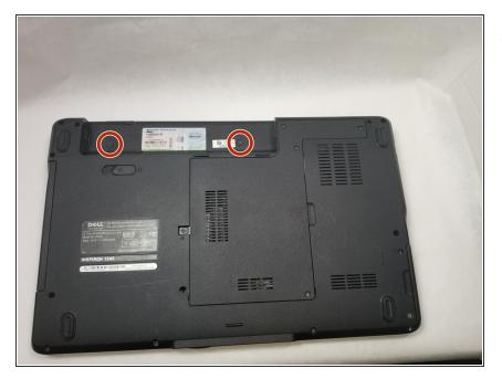
Once the battery has been removed, take out the two screws (3mm Phillips #1) beneath it. These screws hold the center control cover in place.
