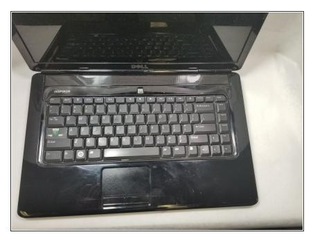
• Flip the laptop back over to the front and push the screen open as far as possible.
