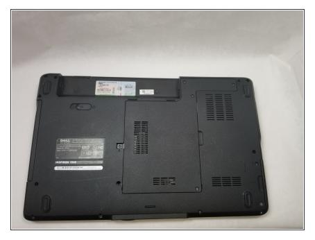
• Slide the battery completely out of the bay.
