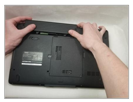
Slide the release latch while simultaneously pulling the battery outwards.
