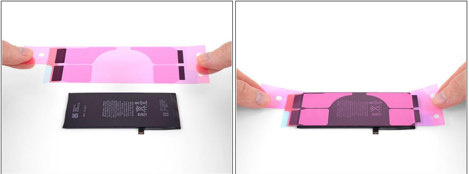
**i** Once the adhesive sticks to the battery, you can't peel it off or reposition it—if you make a mistake, you'll have to start over with fresh adhesive strips.
