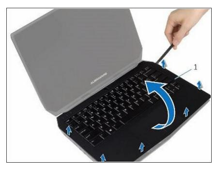
Using a plastic scribe, pry up along the edges of the palm-rest assembly.
