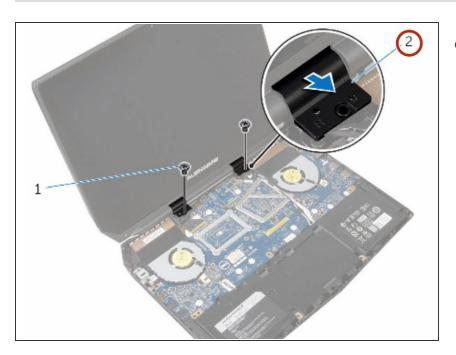
Slide and lift the hinge caps off the display hinges.
