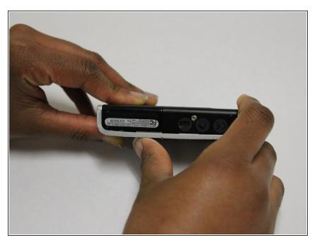
Turn the camera to the bottom and find the battery access door on the left side.
