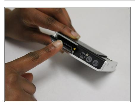
Remove the battery and replace with a new one.
