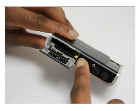
Push the yellow tab to eject the battery.
