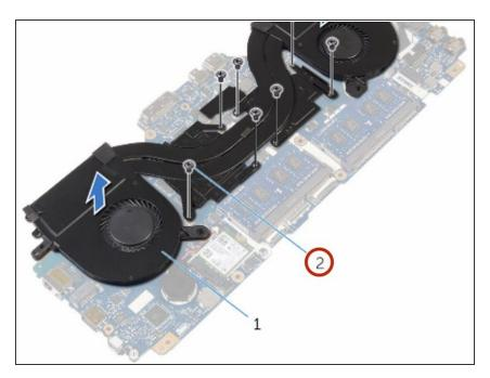
Remove the screws that secure the heat-sink assembly to the system board.
