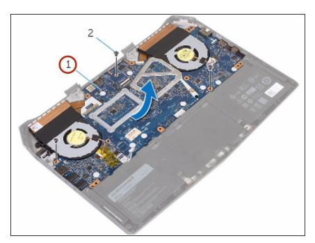
• Slide and lift the system-board assembly.
