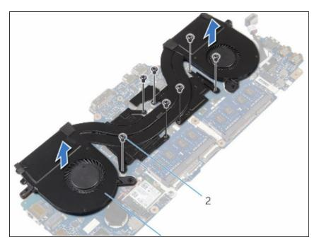
Align the screw holes on the NEW heat-sink assembly with the screw holes on the system board.
