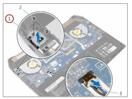
• Lift the power-adapter port bracket off the power-adapter port.
