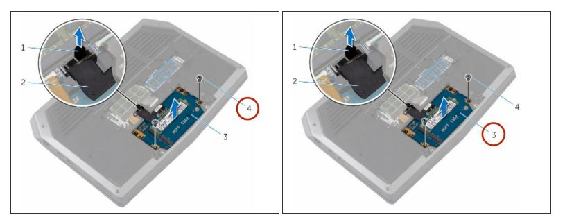
Align the screw holes on the solid-state drive assembly with the screw holes on the computer base.
