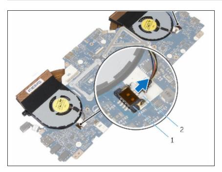
• Connect the fan cables to the connectors on the system board.
