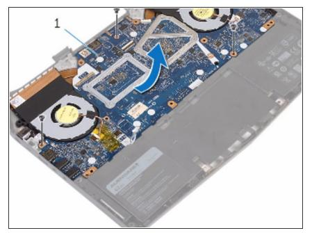
• Align the screw hole on the poweradapter port bracket with the screw hole on the power-adapter port.
