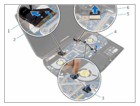
Adhere the adhesive tapes that secure the antenna cables to the system board.
