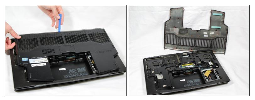
• Use the iFixit opening tool to lift the bottom cover off.
