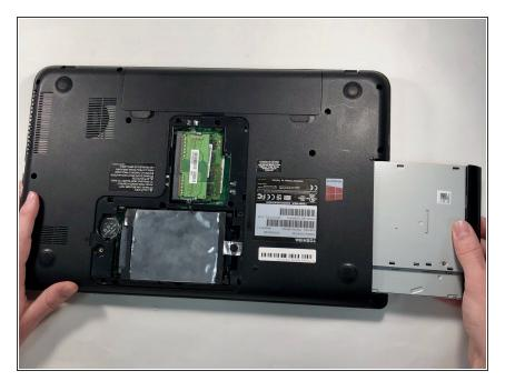
• Remove the disc drive from the device.
