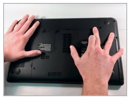
Press down with your fingers while also applying a sliding motion on the latch buttons near the battery on the underside of your laptop.
