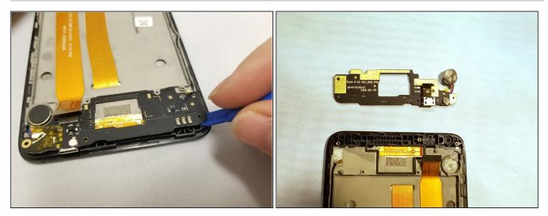
• Using the black spudger, pry off the board the USB charging port is attached to.
