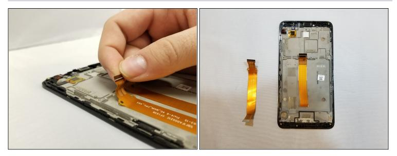
Do not damage the ribbon cable; you'll need to save it for reassembly.
