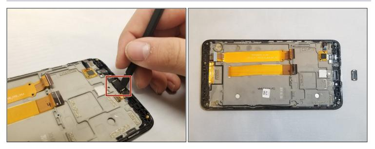
The earpiece speaker is heavily glued onto the device. Make sure you're reaching far enough down before you start prying.
