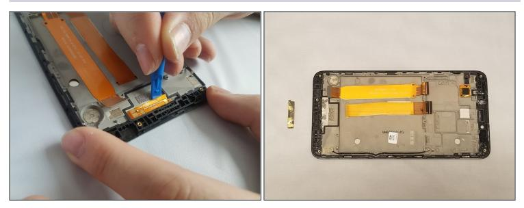
You will need to save the antenna to reapply to the new assembly.
