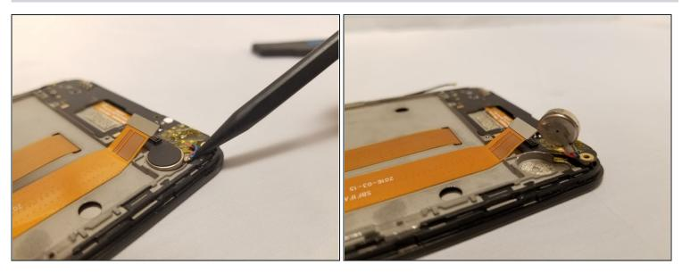
A Be sure that you're reaching down far enough into the crack before you begin prying the vibrator up, or you could break it.
