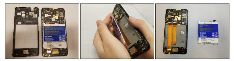
• Remove the blue battery by lifting it straight up, or by gently turning the phone over into your palm and catching the battery as it comes out.
