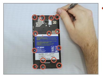
Using a Phillips #000 screwdriver, remove the fourteen 3mm screws that connect the housing and the battery.
