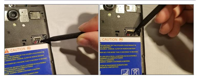
• Disconnect the battery connector flex cable by sliding the black spudger under the wires and carefully prying up the entire terminal casing.
