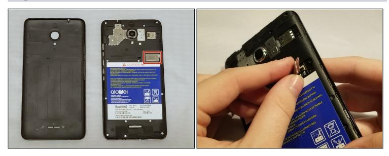
• Remove the metal bracket covering the battery connector flex cable. Now that it's unscrewed, it should come out easily.
