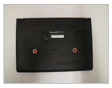
Remove two Phillips Head 5 mm #0 screws holding the backing in place.
