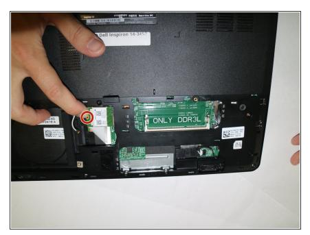
Remove the Phillips Head 3 mm #0 screw that is holding the wireless card in place.
