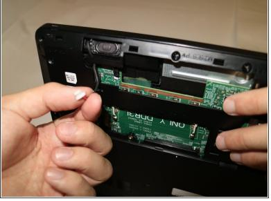
Using your fingertips remove the speaker cable from the motherboard by pulling the white connector away from the socket.
