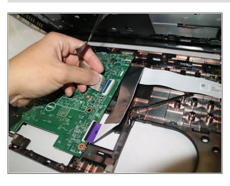
Disconnect the keyboard cable from the motherboard by lifting the black latch and pulling the cable out of its socket.
