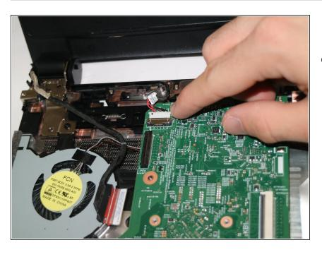
Remove the power adapter cable from the motherboard by sliding the cable out of its socket.
