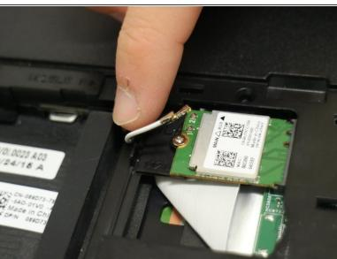
Remove the white and black antenna cables from the wireless card.
