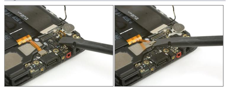
Use a spudger to disconnect the headphone jack and the loudspeaker flex cables.
