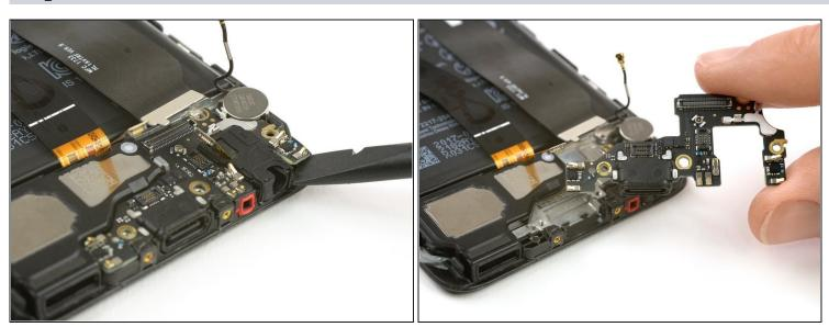
$\Delta$  Do not damage any components sitting on the charging board while removing it.
