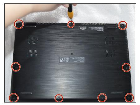
Using a Phillips #0 screwdriver, remove all nine of the screws along the outside of the bottom of the laptop.
