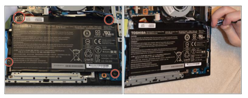
Using the Phillips #0 screwdriver, unscrew each of the four screws holding the battery in place.
