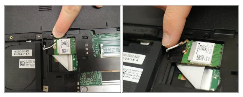
• Remove the white and black antenna cables from the wireless card.
