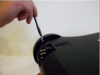
Unscrew both screws near the wheels.
