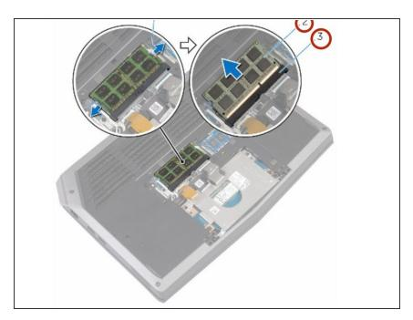
Using the new memory module, align the notch on the memory module with the tab on the memorymodule slot.
