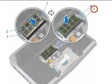
Slide the memory module firmly into the slot at an angle and press the memory module down until it clicks into place.
