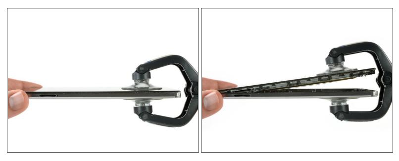
Use an iSclack or a suction handle in the bottom area of your phone to separate the display unit from the rear panel.
