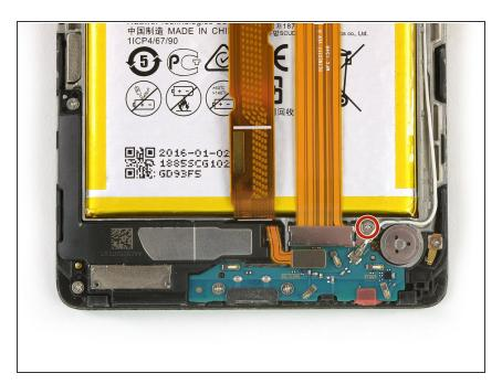
Remove the Phillips #00 screw that holds down the interconnect cable bracket.
