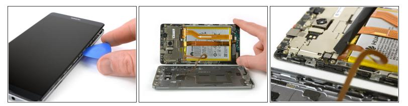
• Use an opening pick to fully separate the clips, releasing the phone.
