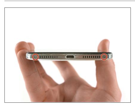
Remove the Torx T2 screws from the bottom of the phone
