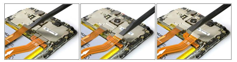
Use the flat end of a spudger to disconnect the display, daughterboard interconnect, and battery cables.
