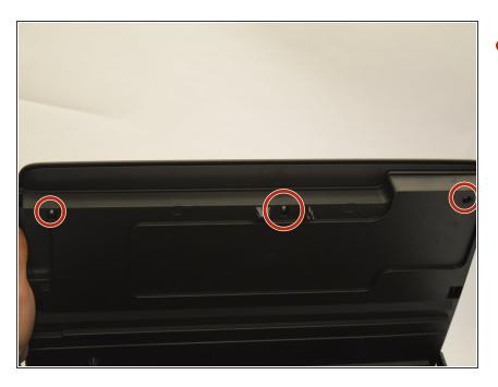
Remove the three 11.5 mm screws with a T10 bit.
