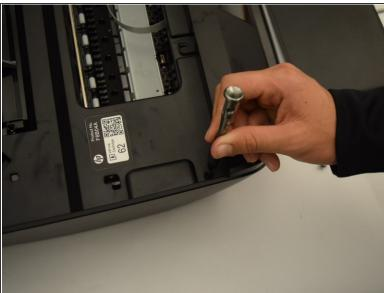
Remove the 12 mm screws on the left side of the printer with a T10 bit.
