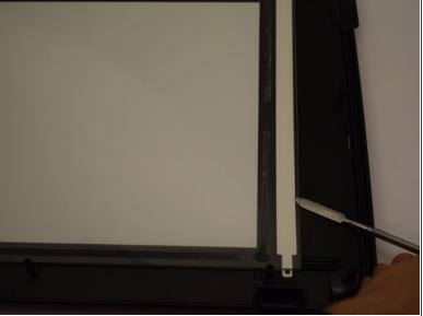
Pry the old scanning glass up with a metal spudger.
