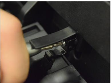
Remove the 11.5 mm screw with a T10 bit to release the spring-loaded hinge.
