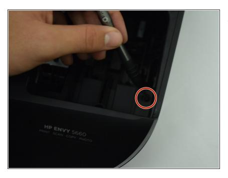
Unscrew the black 11.5 mm screw closest to the front right corner using a T10 screw bit.
