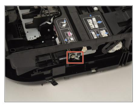
Remove spring from the side of the print head rail using a metal spudger.
