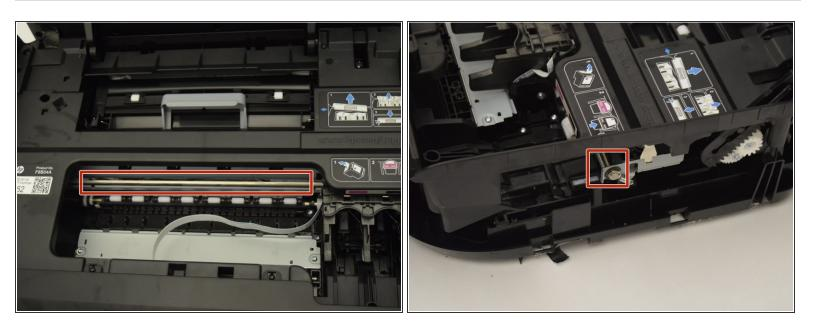
Push the metal rail the print head rests on inwards to remove it from its bearings.
