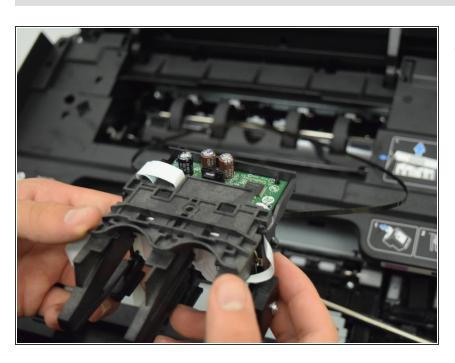
Remove the print head from the metal rail by sliding it off the rail.
