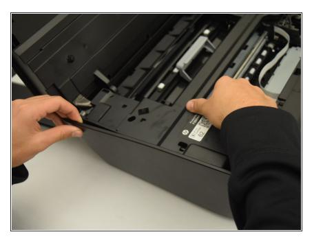
Remove right side of the printer using a plastic opening tool or metal spudger.
