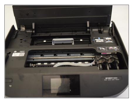
Open the printer so that the underside of the scanner is showing.
