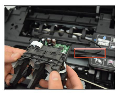
Remove the belt from the back of the print head using a metal spudger.
