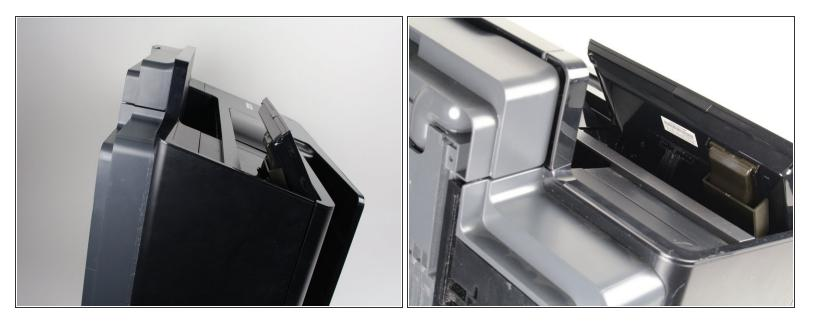
Place the printer on its back and rotate the display clockwise to gain access to the underside of the display.
